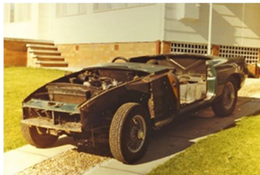
Stripped bare, to chase rust.
