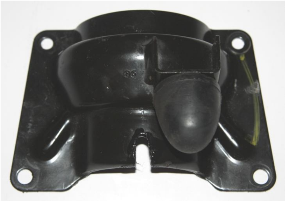
Modified spring unit retainer showing the added slot to facilitate ride height adjustment.
