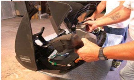
Remove from the dash any mechanical or electronic components that could be damaged during the painting process.
