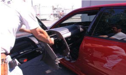
The first step is to remove the major dash components from the vehicle.
